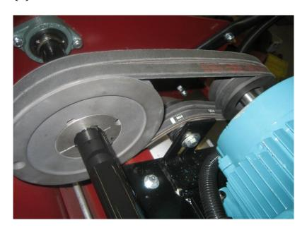
(1) FIG 1 COUNTER SHAFT TO CYLINDER & HYDROSTATIC DRIVE TO DRUM.
